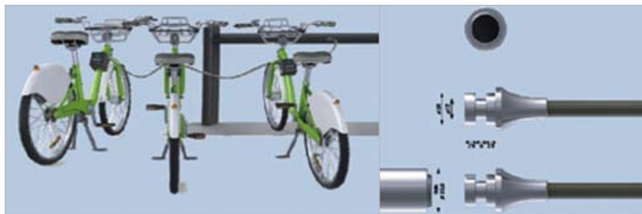
Figure 5.11. A bicycle connection rack and a standard wire lock presented by the Ministry of Security and Public Administration
