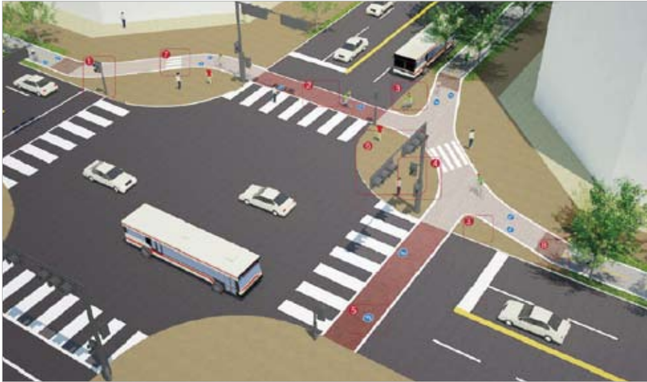
Figure 4.7. An intersection bike path designed to ensure seamless bike traffic
