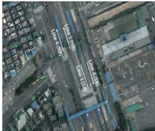
from Line 3 requires attention to go the right direction. The width of the stairs connecting the two lines is insufficient, which causes bottlenecks during rush hours.
