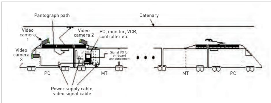
**Figure 6.9** Pantograph monitor camera
