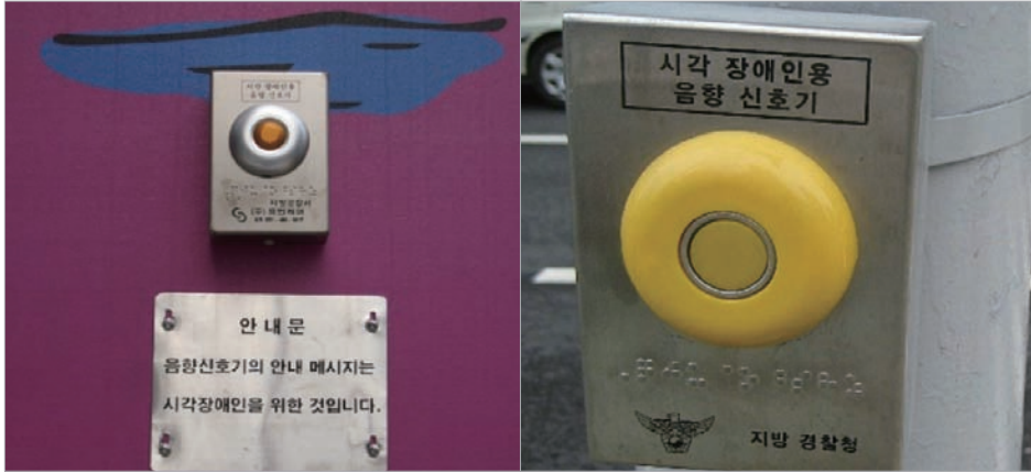
Figure 6.3. Audible signals to assist visually impaired persons
