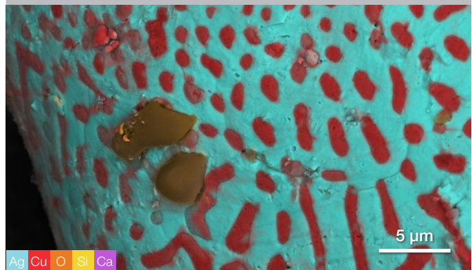
Microstructure of copper-silver alloy revealed with ColorSEM technology. Silicate contamination is immediately recognized when inspecting samples with live compositional imaging via ColorSEM.
